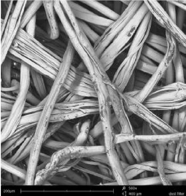
Dust filter taken at 500x magnification (Field of view is 400 µm).
