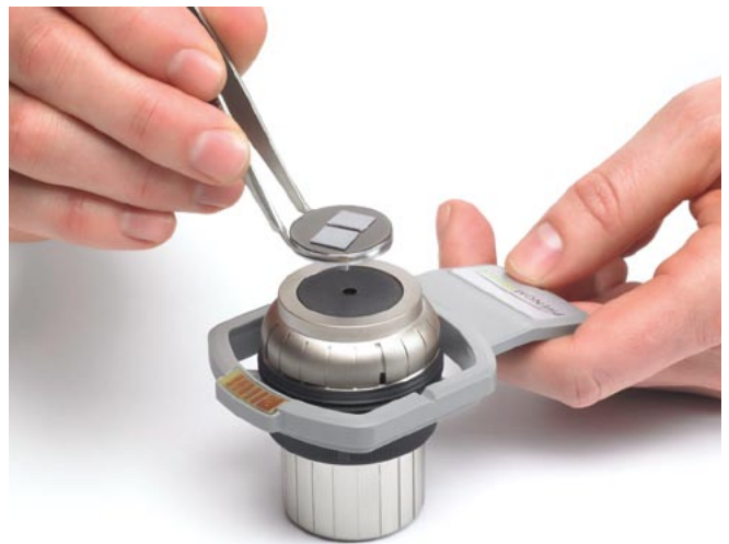
Figure 10: Inserting pin stub in charge reduction sample holder.
