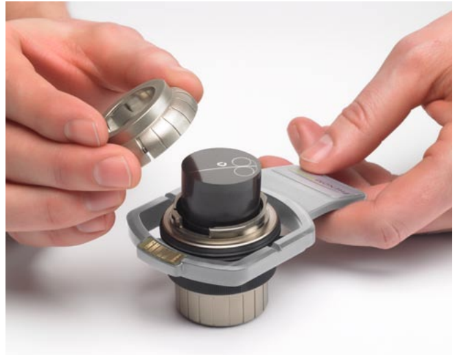
Figure 9: Inserting resin mount in metallurgical mount charge reduction sample holder.
