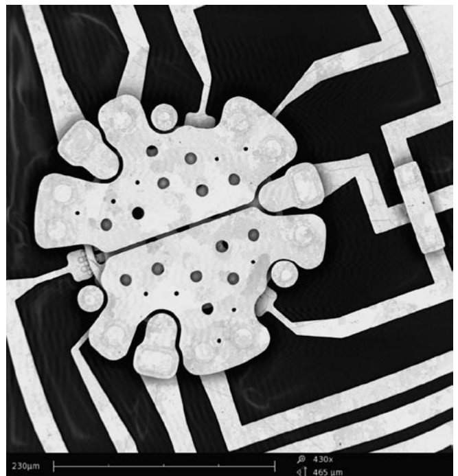
Figure 5: Micro-electronic device. Imaging can provide quality control of wire surfaces and connections.
