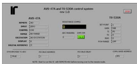
A LabView Application Example combines the AVS-47 and TS-530A into a single virtual instrument.
